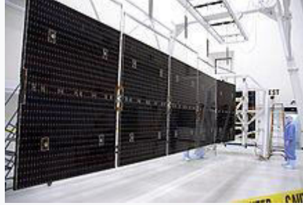
Dawn's 10 kW triple-junction gallium arsenide solar array at full extension
